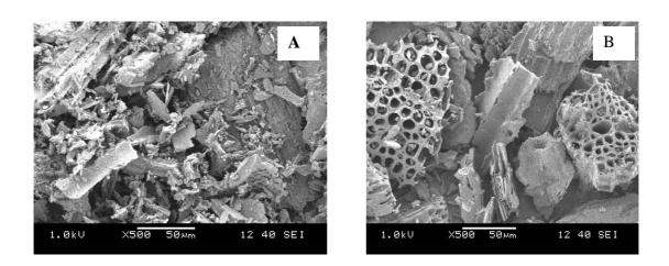
Figure 7. SEM images of OSC before (A) and after (B) adsorption of CR
