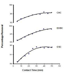
Figure 10. Effect of contact time on the extent removal of CR
