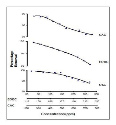
Figure 4. Effect of initial concentration on the extent removal of Congo red dye
