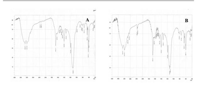
Figure 6. FT-IR spectra of Congo Red before and after adsorption on EOBC
