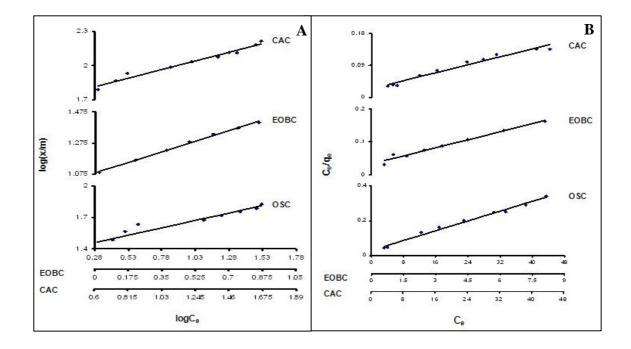
Figure 9. Freundlich (A) and Langmuir (B) adsorption isotherms for the removal of CR various carbons
